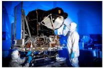
In addition to the instrument (OLI-2), Ball designed and built the cryocooler that will keep Landsat 9's Thermal Infrared Sensor 2 (TIRS-2) chilled to a frigid 40 Kelvin (-388 F). The TIRS-2 instrument, designed and built by NASA Goddard Space Flight Center, measures thermal radiance emitted from the Earth's surface.
