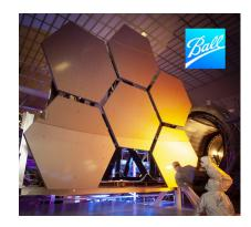
To make this possible, Ball Aerospace worked with NASA's Goddard Space Flight Center and Northrop Grumman, the prime industry partner, to innovate the 25 square-meter (~269 square feet) mirror system consisting of 18 beryllium mirror segments working together as one mirror. It will be the largest mirror and the first segmented telescope ever deployed in space, operating at the extremely cold space temperature of -406° F (30K) necessary for infrared imaging of distant stars and galaxies.
