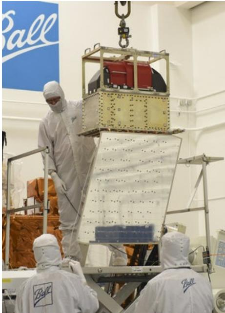
The Advanced Technology Microwave Sounder (ATMS) was the final instrument to be integrated onto the JPSS-1 satellite, scheduled to launch in early 2017. The sounder will continue to provide the same high quality observations currently available from the NOAA/NASA Suomi NPP satellite and necessary to retrieve profiles of atmospheric temperature and moisture for civilian operational weather forecasting as well as continuity of these measurements for climate monitoring purposes.
