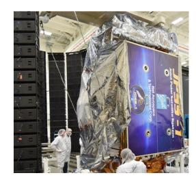
testing from July through early fall. The thermal vacuum testing will expose the satellite and its five instruments to the extreme temperatures experienced in space. A pre-shipment review is scheduled to be held in the fall prior to the spacecraft's shipment to California's Vandenberg Air Force Base for its planned early 2017 launch.
