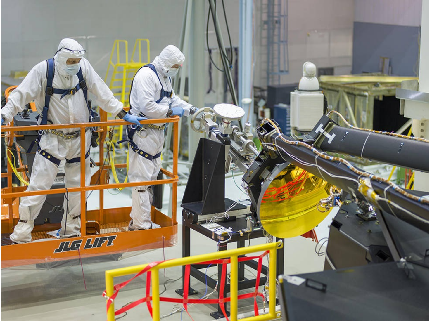
Engineers installing the secondary mirror on the Webb telescope. Credit: NASA/Chris Gunn
