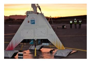
World View has developed Stratollites, a new category of above-earth vehicles that are high-tech balloons offering long-duration, persistent flight above specific geographical areas of interest. Stratollites, as the name suggests, operate in the stratosphere and can maintain station and directionally navigate. They utilize a proprietary method of altitude control to channel directional wind patterns at various altitudes.
