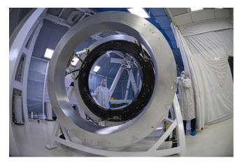
Ball teamed with Arizona Optical Systems (AOS) to build the lens assembly, which consists of two large refractive lenses, named L1 and L2, and the precision structure that will be used to mount the lens assembly to the LSST camera.
