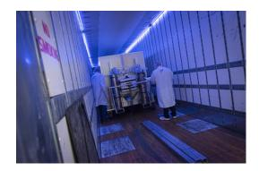
The OMPS instrument observes stratospheric ozone and measures its concentration as it varies with altitude. It is a three-part hyperspectral instrument, which includes a Nadir Mapper that will map global ozone with about 50-km ground resolution, a Nadir Profiler that will measure the vertical distribution of ozone in the stratosphere and the NASA-provided Limb Profiler that measures ozone in the lower stratosphere and troposphere with high vertical resolution.
