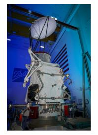
At the heart of the WSF-M payload is the Ball-built MWI sensor that takes calibrated passive radiometric measurements at multiple microwave frequencies to measure sea surface winds, tropical cyclone intensity and additional
