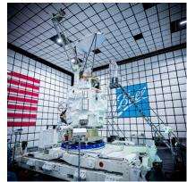
As the prime contractor on the project, Ball Aerospace designed, built and integrated the spacecraft bus, ground data processing software and the Microwave Imager (MWI), the primary instrument on the satellite that uses passive radiometric measurements at multiple microwave frequencies to collect environmental data. The satellite will also host a government-built Energetic Charged Particle (ECP) sensor that will provide space weather measurements in low-Earth orbit.
